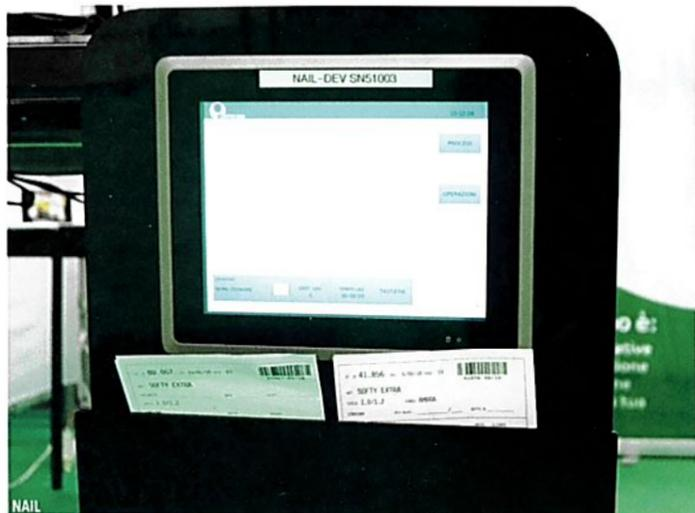
A simple but effective device to be applied on board the machine that allows tracking the progress of production on any type of plant. It is called NAIL and was developed by Center 2000, an IT company that has been operating for more than 30 years in the tanning district of Santa Croce sull'Arno.
